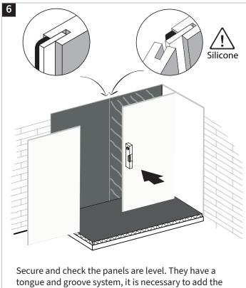
tongue for fitting the joint and add silicone, as image
