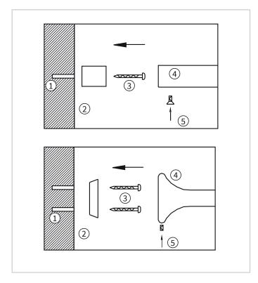
Corresponding to the hole of the small plate (2), drill and put into the wall the screw wall plug (1). Then with the screw (3) fasten the small plate on the wall.
