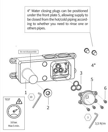
Suggestions for flushing out and water tightness installation test
